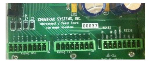
Figure 13 Analog I/O Wiring Terminals
