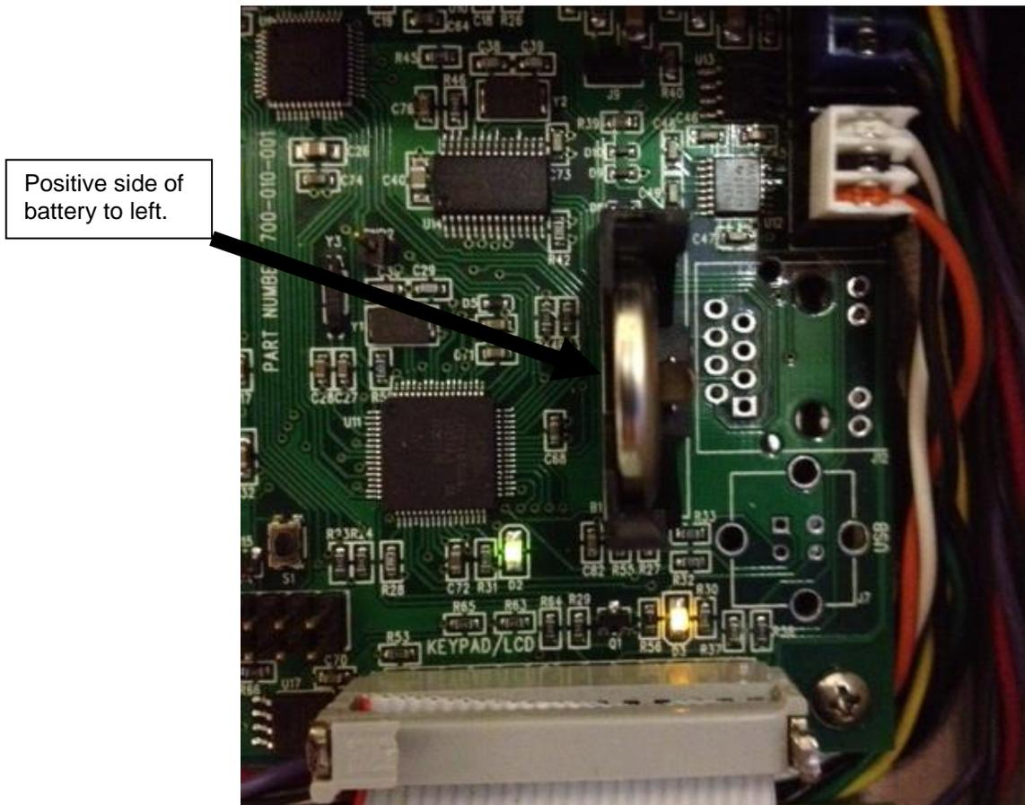
Figure 20 Battery Installation
