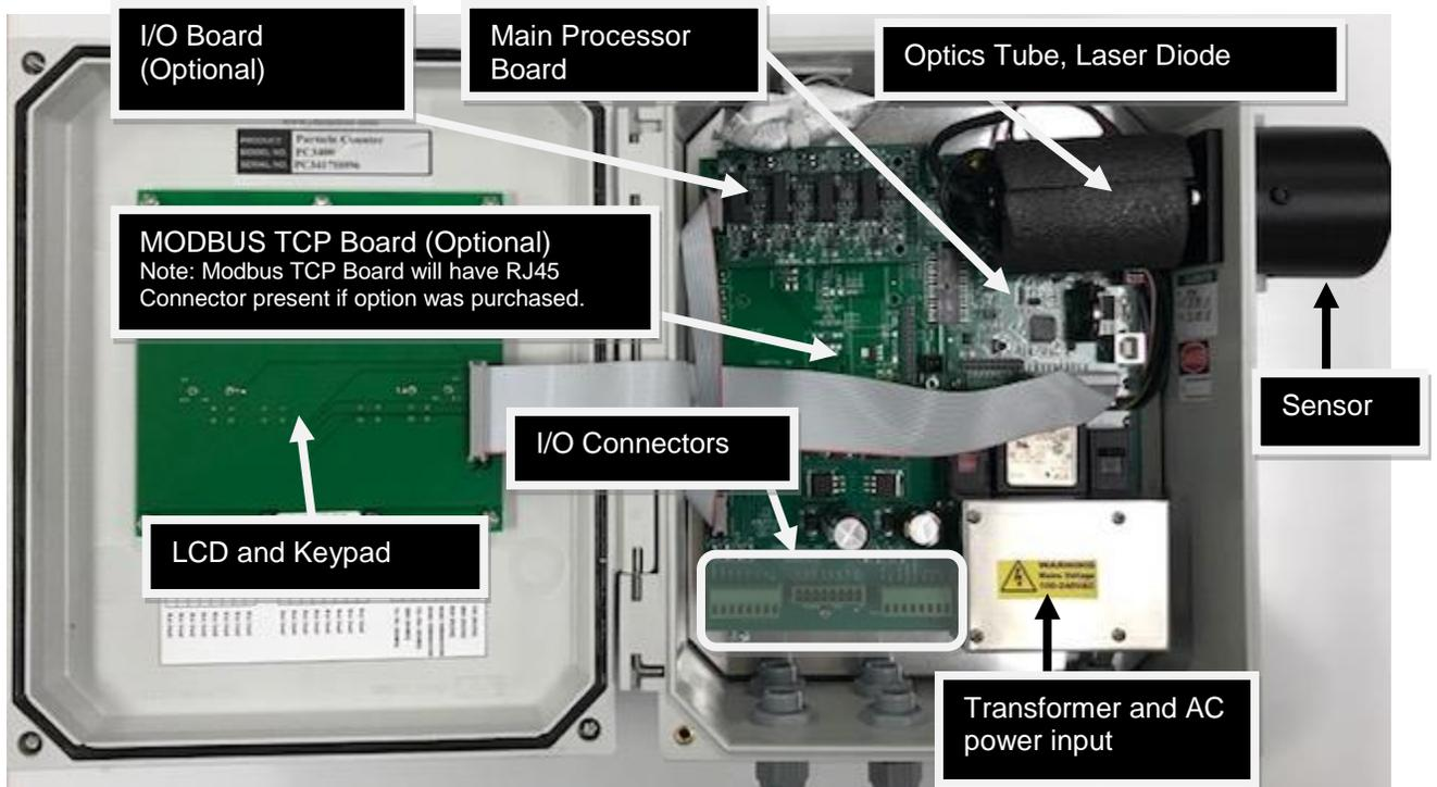
Figure 3 System Components
