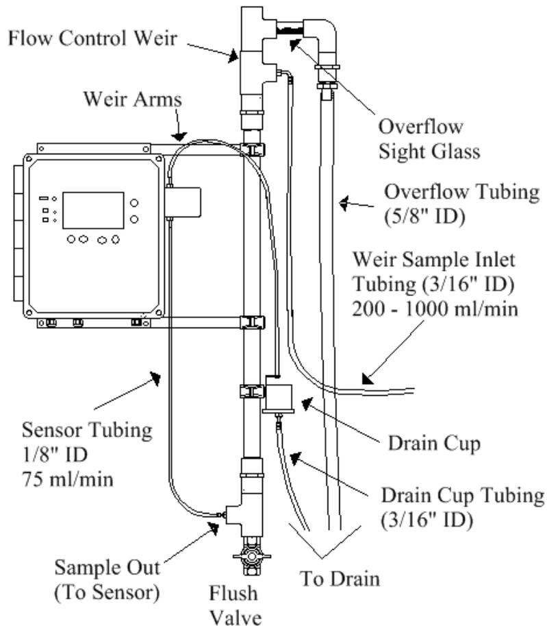
Figure 4 PC3400 and Flow Control Weir Plumbing
