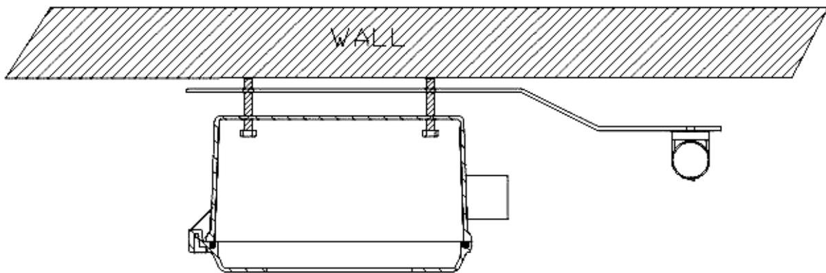
Figure 7 Mounting with Weir Arms – Top View
