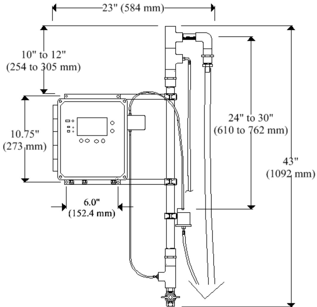
Figure 6 Mounting Dimensions
