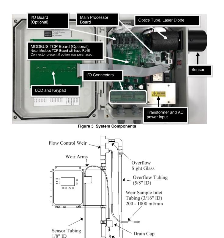
Figure 4 PC3400 and Flow Control Weir Plumbing
