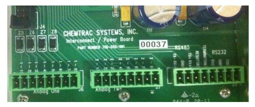
Figure 13 Analog I/O Wiring Terminals
