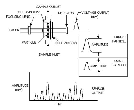
Figure 1 Light Obscuration Measurement (Diagram 1)
