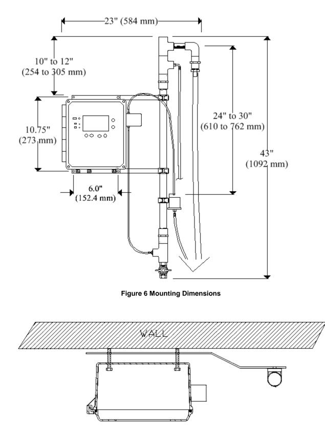
Figure 7 Mounting with Weir Arms – Top View
