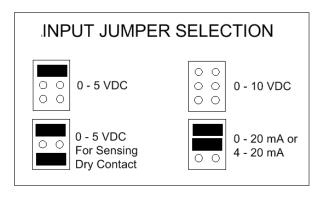
Figure 14 Analog Input Type Jumper Selection
