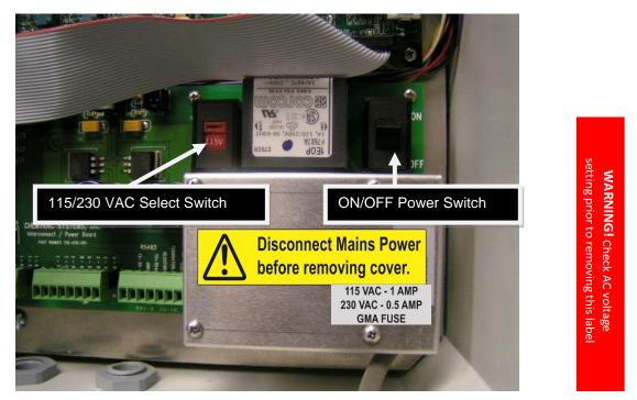
Figure 8 115/230V and Power Switches
