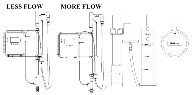
Figure 17 Sensor Flow Rate Adjustment
