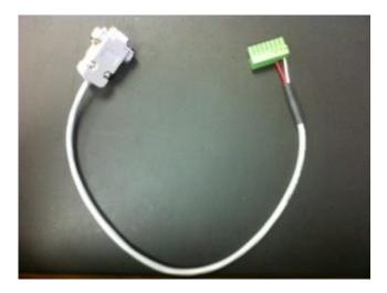
Connect the DB9 end of the download cable to a Com port on your PC. Alternatively, if your computer only has USB ports, you will need to connect the DB9 connector to a USB to Serial converter that gets plugged into a USB port. Contact Chemtrac for recommended USB to Serial converters.
