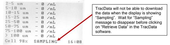
**Note:** Make sure the PC3400 display is not in the User Menu. TracData cannot communicate to the PC3400 if it is in the User Menu mode.
