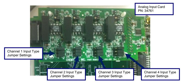
Figure 15 Optional Analog Input Card
