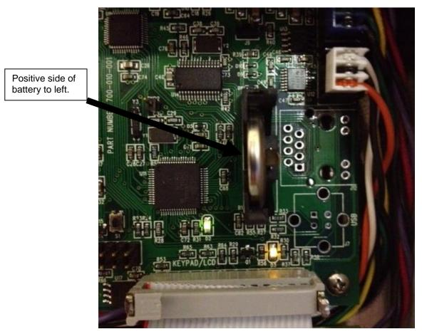
**Figure 20 Battery Installation**
