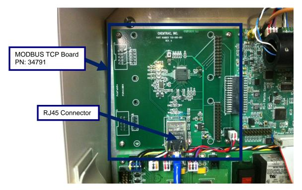
Figure 12 Optional MODBUS TCP Communications
