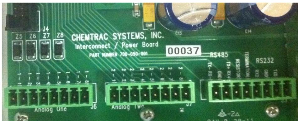
Figure 13 Analog I/O Wiring Terminals
