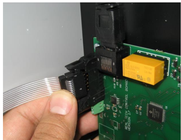
Figure 5.9: Attach cable to control board
