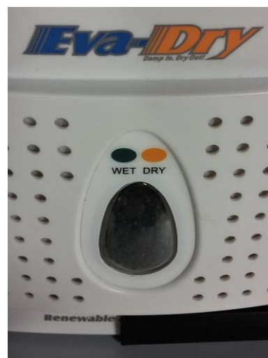
Figure 13.2: Dehumidifier Bead Color and Moisture Saturation
