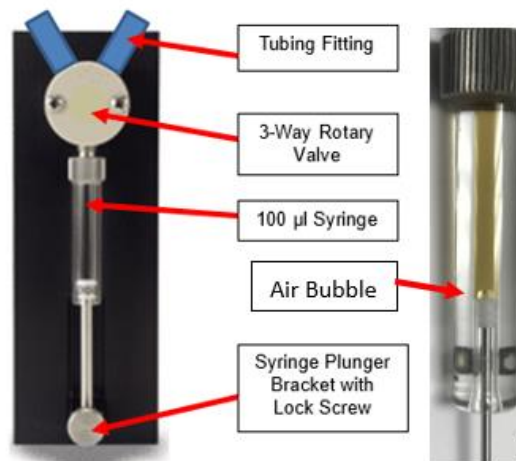
Figure 6 – Syringe Pump Components
