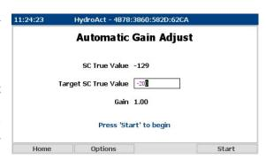
to edit the Target SC True Value. Ensure the Start button turns gray as this indicates you are in edit mode. Use the navigation buttons to set the Target SC True Value to -200, which is the recommended setting for most applications. Adjust to a higher value (e.g., -300) for more sensitivity or a lower value (e.g., -100) for less sensitivity to chemical feed changes. Ensure both the SC True Value and Target SC True Value are negative numbers before pressing Start.
